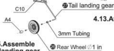
4.12. Glue to vertical stabilizer as shown
