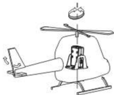
Helicopter (Yaw Stabilization) RX ⇔ PG-02 ⇔ Rudder Servo
